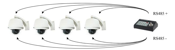
Run a cable individually from the RS485 + / - ports on the joystick to the corresponding wire on each of the cameras. This is ideal for cameras that are placed far apart from one another but are near the joystick.
