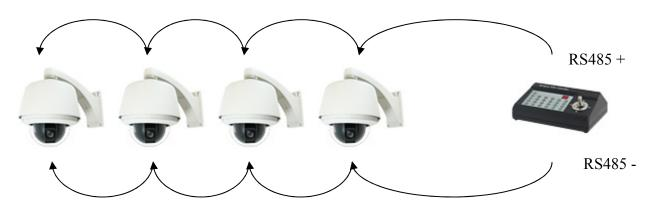
Run a cable from the RS485 +/- ports on the joystick to the corresponding wires on the first camera. Then run a cable from the RS485 +/- wires on the first camera to the second, and from the second to the third, etc. This is ideal for cameras that are spaced close together to each other, but may be far away from the joystick individually.
