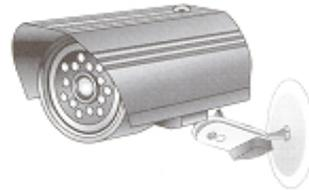
1. Fix the bracket on wall or ceiling, then fix the camera on the bracket.
