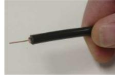
Step 2: Then strip away the black outer jacket so you have 1/4" of the shielding exposed. Do not allow any of the copper shielding to touch the center conductor.
