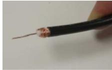
Step 3: Insert the cable into the fitting and gently find the hole for the center conductor before you press the fitting onto the wire. Now just twist the fitting onto the wire while firmly pressing down until the fitting is firmly on the cable.
