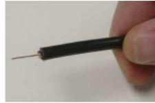
Step 2: Then strip away the black outer jacket so you have 1/4" of the shielding exposed. Do not allow any of the copper shielding to touch the center conductor.
