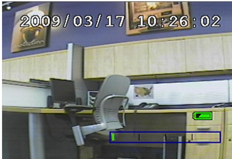
The Battery Life Indicator will show as a green battery on the screen. The more of the battery is filled in, the more charge the battery has. When power is lost to the camera, the indicator turns white. The camera can function for up to 2 hours on battery power alone.
